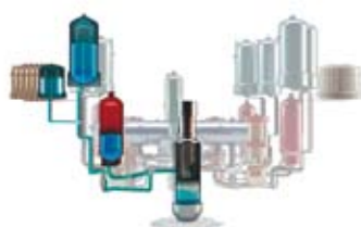
Systems of passive core filling (HT-2, HT-3)
